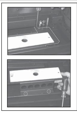
**Figure 6.2** Remove the burner support by *loosening* the left screw on the pilot tower, and removing the two screws on the front side of the burner neck support.
